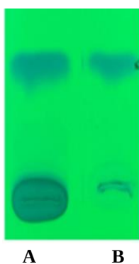
Fig. 2. TLC plate under UV 254 nm: (A) Green tea extract and (B) Epigallocatechin standard.
